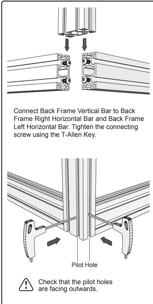
Connect Back Frame Vertical Bar to Back Frame Right Horizontal Bar and Back Frame Left Horizontal Bar. Tighten the connecting screw using the T-Allen Key.
