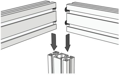
Connect Back Frame Left Horizontal Bar and Back Frame Right Horizontal Bar to the Back Frame Vertical Bar. Tighten the connecting screw using the T-Allen Key.
